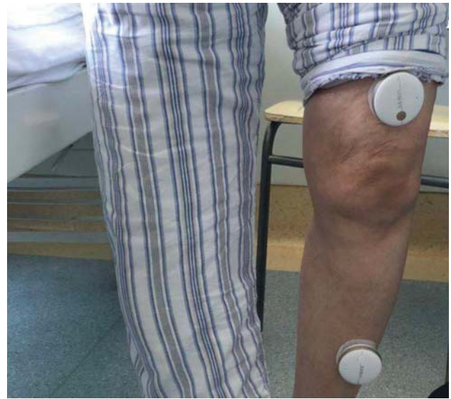
Fig. 3 Measurement of the knee joint angles using two data acquisition modules.
